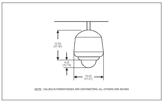
Figure 8. BB08E120 and BB08E211 Dimension Drawing
